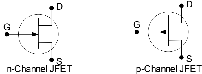
Drawing 17: Schematic Symbols for J-FETs
